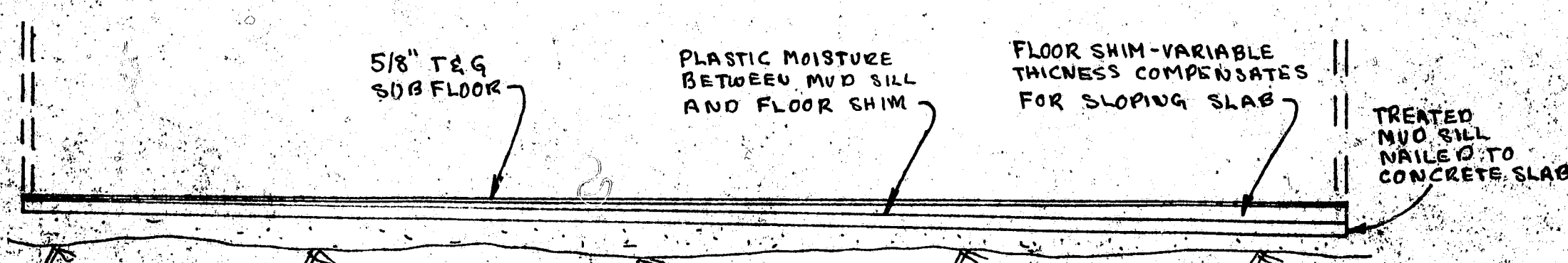
EXISTING FLOOR x-section 1/2"=1'
